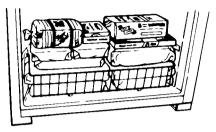
**Basket** – Store heavy and bulky packages here. Basket should be in place at all times for proper air circulation.
